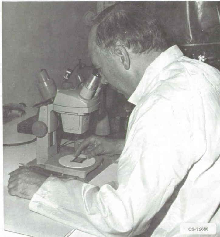
Figure X-20. - Optical inspection of microelectronic modular assembly.
